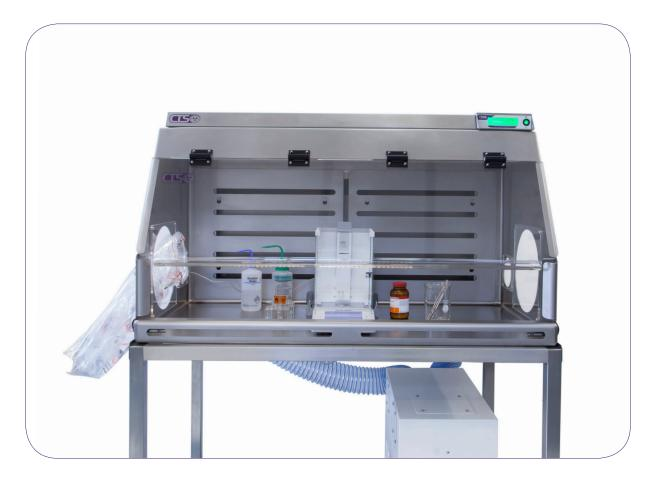
The HiPo VBETM is specifically designed for the weighing and manipulation of high potency powders.
