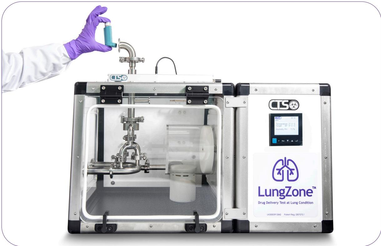
The LungZone™ provides a controlled temperature and humidity environment (37°C - 95% RH) for testing inhalation drugs, replicating climatic conditions within the lung during the respiratory cycle.
