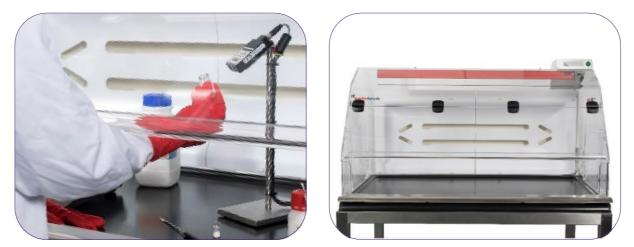
Activities such Lyophilisation, Spray Drying, Milling and Micronisation can create static problems with powders making them difficult to weigh accurately in small quantities. Ionizing bars can be used to neutralize the area close to them in order to help reduce the effects of static.
