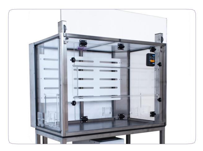
CTS LEV (Local Exhaust Ventilation) series of enclosures are designed and built specifically to the customer's requirements and can be used to contain automation equipment, particle size analysis, small scale synthesis, sieving and sample handling.
