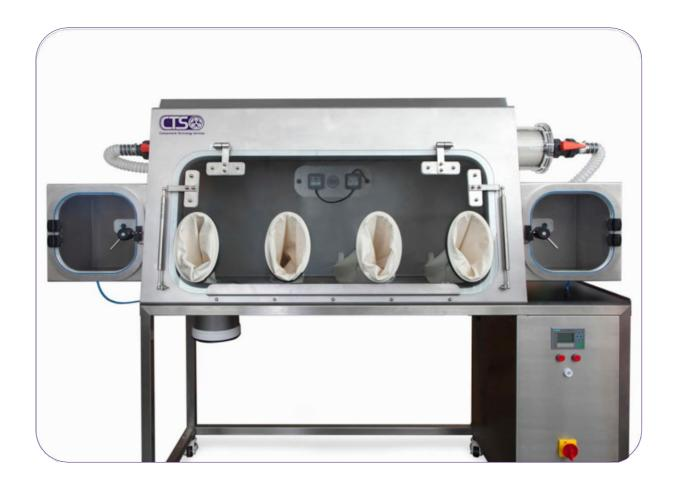
CTS Powder Handling Isolator systems provide a safe controlled environment for weighing and manipulation of high potency drugs with OEL's less than 30 ng/m<sup>3</sup>.
