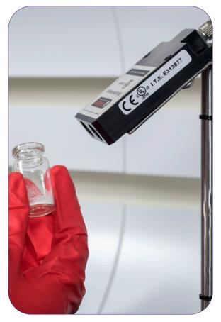
Activities such Lyophilisation, Spray Drying, Milling and Micronisation can create static problems with powders making them difficult to weigh accurately in small quantities. Ionizing bars can be used to neutralize the area close to them in order to help reduce the effects of static.
